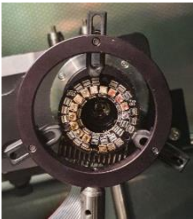
Figure 3. Illumination of the system. (left) Circular board of the LEDs. (right) Spectra of the LEDs, normalized to 1.
