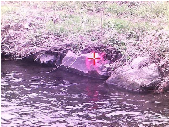
Disto proof images of a measurement performed for a GCP and during the measurement of the cross-section.
