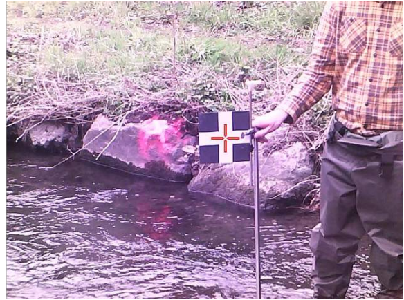
Disto proof images of a measurement performed for a GCP and during the measurement of the cross-section.
