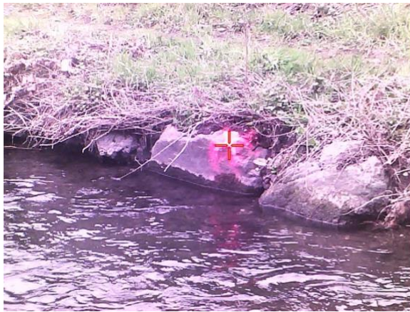
Disto proof images of a measurement performed for a GCP and during the measurement of the cross-section.
