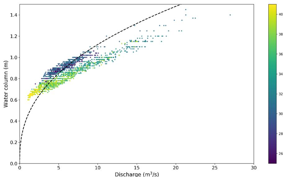
**Figure 6. Water level and discharge data measured for the 2018 melting season color-coded with the calendar week before the correction for the de-rating event. Note the de-rating event occurring at the beginning of the calendar week 32.**
