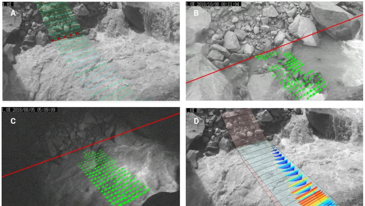
**Figure 3. (A) Bathymetry projected on an image of the canyon (green) and optically detected water level (red). (B) Measured water level and flow field under low flow conditions. (C) Water level and flow field obtained for a night measurement. (D) Horizontal and vertical profiles of the streamwise velocity component used for the discharge computation.**
