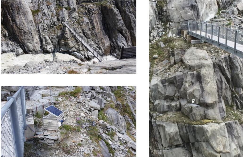
**Figure 1.** Canyon in which the measurement system is installed (top). Camera located below the bridge (right). Solar panel and box containing the fuel cell, processing and transmission units (bottom).
