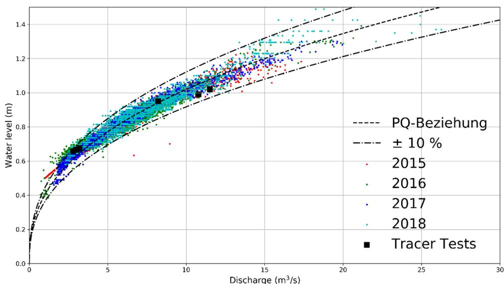
**Figure 5. Measured water level plotted as function of the measured discharge for the melting seasons 2015 to 2018, as well as several tracer tests performed (black dots). The black dashed-line presents a possible rating-curve and the dot-dashed lines represent 10 percent intervals.**
